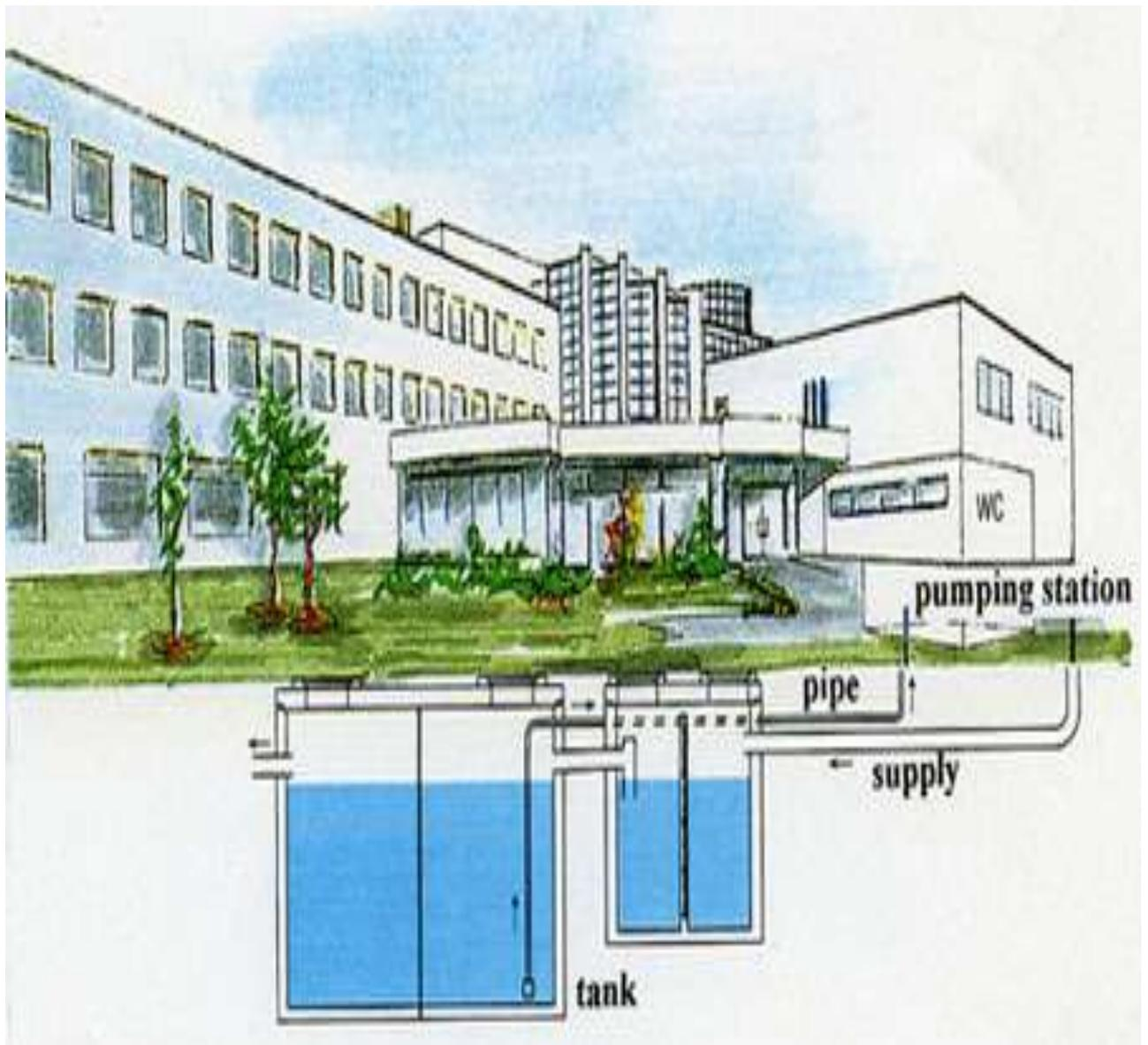
Water is collected through pipes which are connected to the roofs of the entire campus. The collected water is drained through drain system created in the peripheral of the campus. The water is finally collected to rain water harvesting.
